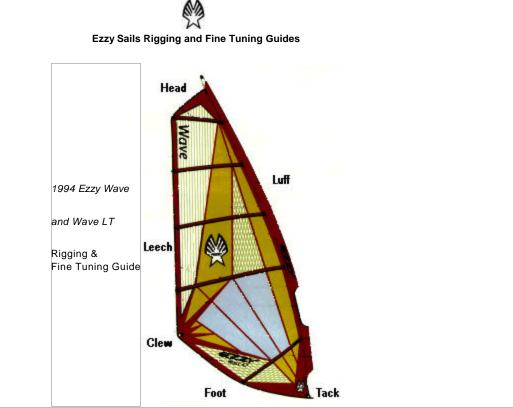
1) Insert the foot batten, then slide the mast through the luff sleeve.
