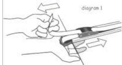
**Quick Tip:** The correct batten tension is when there are no wrinkles running across the batten pocket when the sail is properly downhauled.
