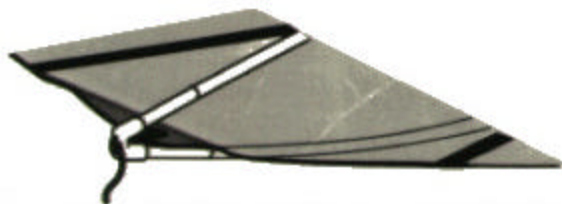
Slight negative outhaul setting for light wind.
