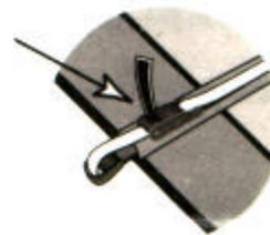
**5) Downhaul the sail until the leech goes loose between battens #2 and #3.** Use the printed marks as a reference. For light wind, the looseness should extend to mark #1. For medium wind the looseness should extend to mark #2 and for strong wind, the looseness should extend to mark #3. At the head of the sail, batten #1 is designed to *always* be very loose. See diagram below:
