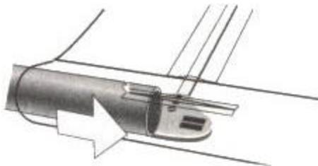
*slide the mast above the cams.*
