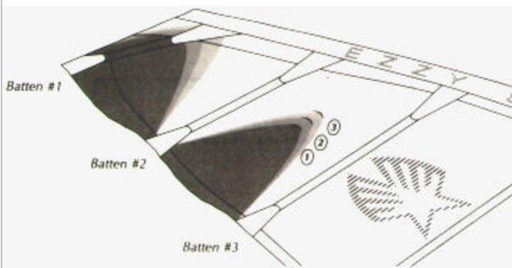
The amount of downhaul tension will vary for different wind conditions: A high-wind setting requires more downhaul tension to loosen the upper leech and give more twist. In lighter wind, the sail needs less downhaul for a tighter leech and better low-end power.
