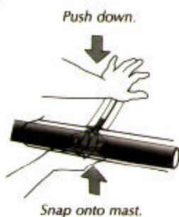
loosened until the Velcro™ touches the buckle. This will allow the cam to slide further from the mast and will make it easier to get the cam onto the mast. Also, make sure the sail is outhauled flat before attempting to snap the cams onto the mast.
