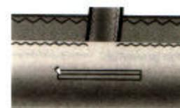
Sleeve is tight when batten is correctly tensioned.
