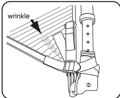
Wrap your downhaul line around the mast base. Tension the tack strap until you get a small wrinkle running out from the corner, then wrap the tack strap over the downhaul line and loop it under itself.
