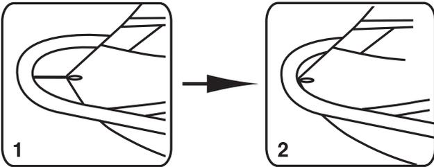
1) With your sail correctly downhauled, adjust your boom length. Hold the sail's clew-cord straight out and adjust the boom-end to meet it (use the short cord for light wind, medium cord for medium wind and long cord for strong wind).
