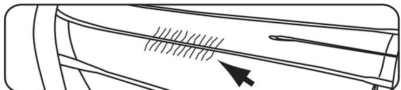
Use the tensioner key, that is stored at the tack of the sail to tension the battens until any vertical wrinkles that extend on either side of the batten pocket are eliminated.
