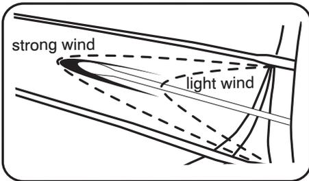
Pull the downhaul and watch the sailcloth slacken by the printed swoosh between battens #2 and #3. For light wind, downhaul until the slackness just reaches the back of the swoosh. For strong wind, downhaul until the slackness extends to the front of the swoosh.
