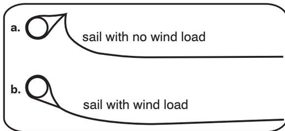
When unloaded, the cross-section of the batten above the boom will look like diagram (a). Loaded with wind, it will look like diagram (b).
