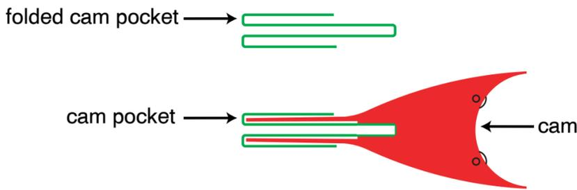
6) Insert the cam and cam pocket into the sail by holding the guide flaps and sliding the cam arm into the openings on either side of the batten stopper. Push the cam all the way until it is fully seated in the sail.
