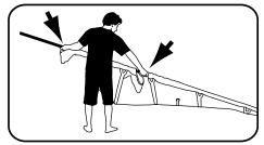
Hold the mast sleeve above the boom cutout and push the mast in with your other hand. It helps to spin the mast. Try not to crease the X film.
