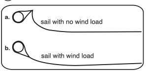
When unloaded, the cross-section of the batten above the boom will look like diagram (a). Loaded with wind, it will look like diagram (b).
