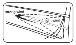
Pull the downhaul and watch the sailcloth slacken by the printed swoosh between battens #2 and #3. For light wind, downhaul until the slackness just reaches the back of the swoosh. For strong wind, downhaul until the slackness extends to the front of the swoosh.
