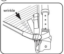
Wrap your downhaul line around the mast base. Tension the tack strap until you get a small wrinkle running out from the corner, then wrap the tack strap over the downhaul line and loop it under itself.
