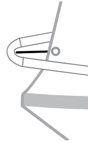
Fig. 3: Adjust the boom length to the outhaul cord.
